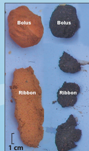
Figure 1: Manipulation of soil for field texturing. The properties of each soil when doing this determines texture.
