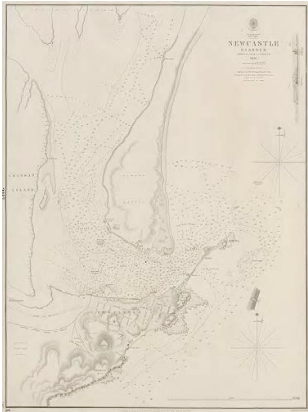
Figure 8.3. Newcastle Harbour, surveyed by Captain I L Stokes, R.N. 1851. This plan shows the limited extent of wharfage in Newcastle in 1851, with a sea wall under construction on the river frontage between Perkins and Watt Streets. It also shows the AA Company railway, A, B and C Pits, miners village and Dangar's preserved meat establishment. Incidentally it also reveals the extent of the Sandhills in Newcastle East and the route of the covered road. It also reveals the "Bathing Head" near the Military Barracks. Source. National Library of Australia. http://nla.gov.au/nla.map-vn3791291-e
