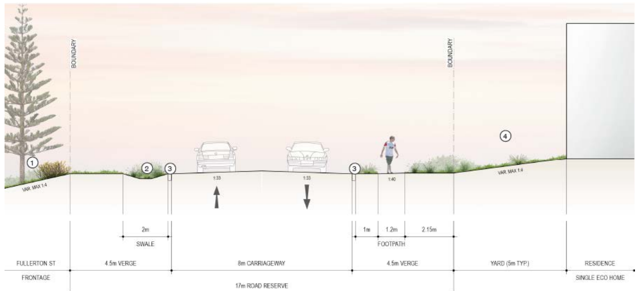
Figure 3 - Road Type 1 Typical Section
