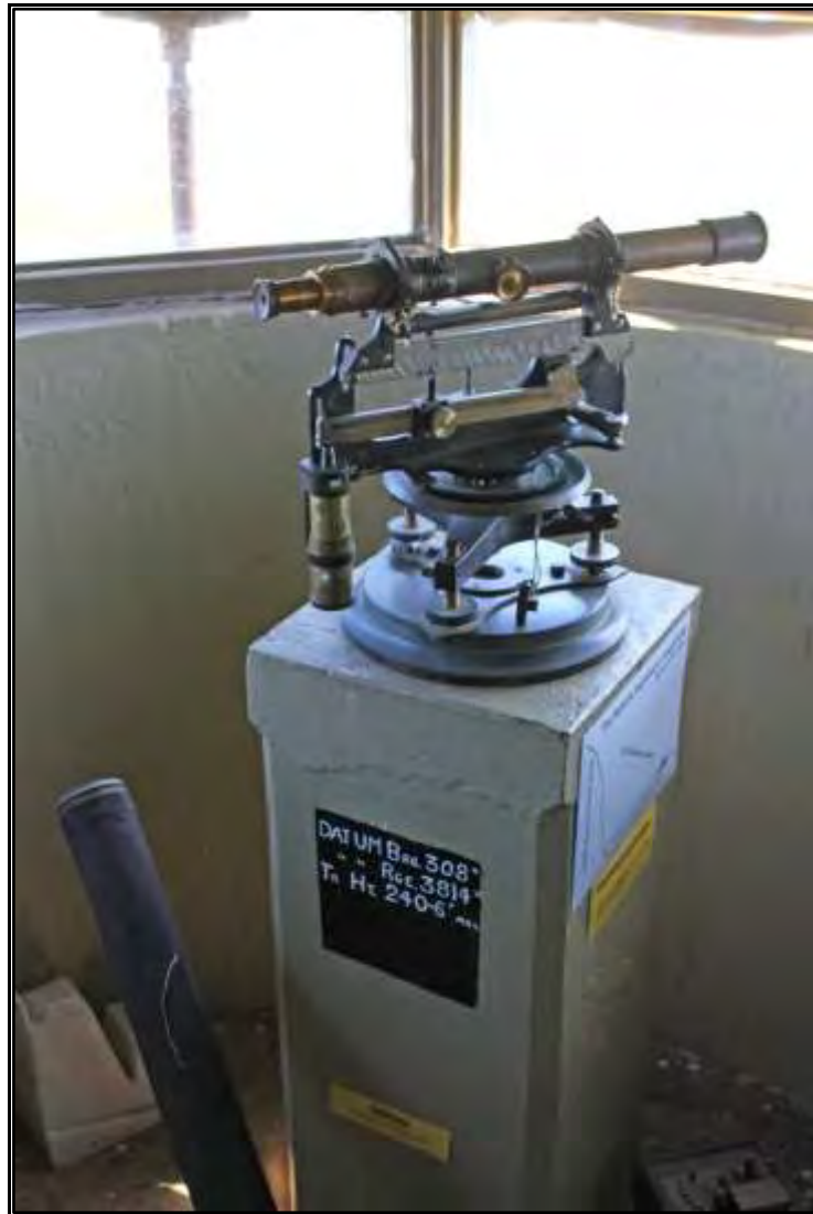
Figure 5: Depression Range Finder restored on concrete mounting Taiaroa Head, Otago, New Zealand (note the datum figures on the mounting for quick reference)
