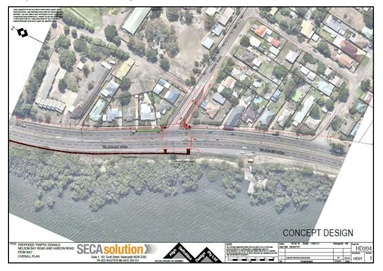
Figure 12.1 - Concept design for Nelson Bay Road and Vardon Road upgrade to traffic control signals
