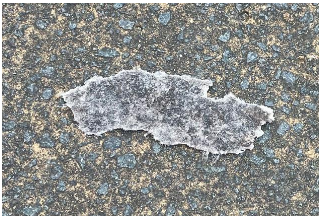
Asbestos debris from the fire. Photo: Hazmat Services
