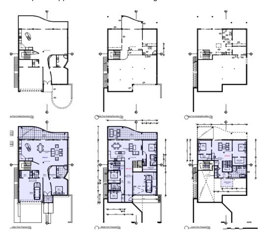
Figure 2 - Existing and proposed floor plans
