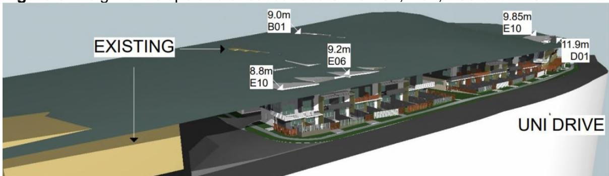
**Figure 6:** Height envelope and exceedances Units E06 and E10
