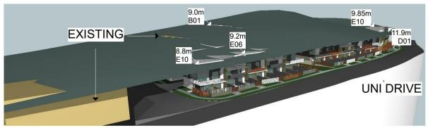
Figure 6 Height Envelope Above Natural Ground Level (o'Connell architecture and design, 2020)
