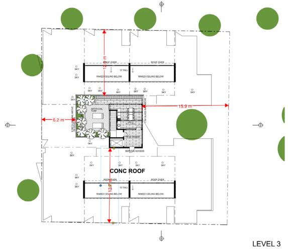
Figure Two – Level Three with setbacks to property boundaries
