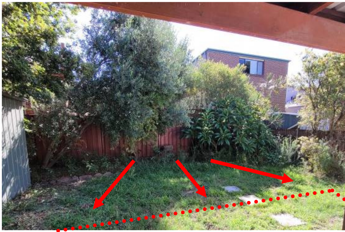
Figure 4 – showing the location of the proposed development in red. The area as highlighted by the arrows are to be retained to protect the TPZ and existing soil levels during construction works. This area is to be cordoned off in order to protect the root plate and canopy.
