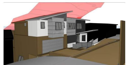
Figure 6 - Computer generated 3D image showing the CoN maximum building height control as viewed from the rear.
