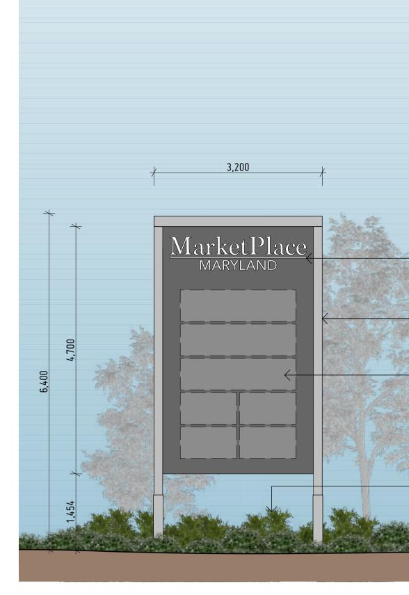
STEEL COLUMN WITH TIMBER INFILL TO MATCH — AWNINGS
