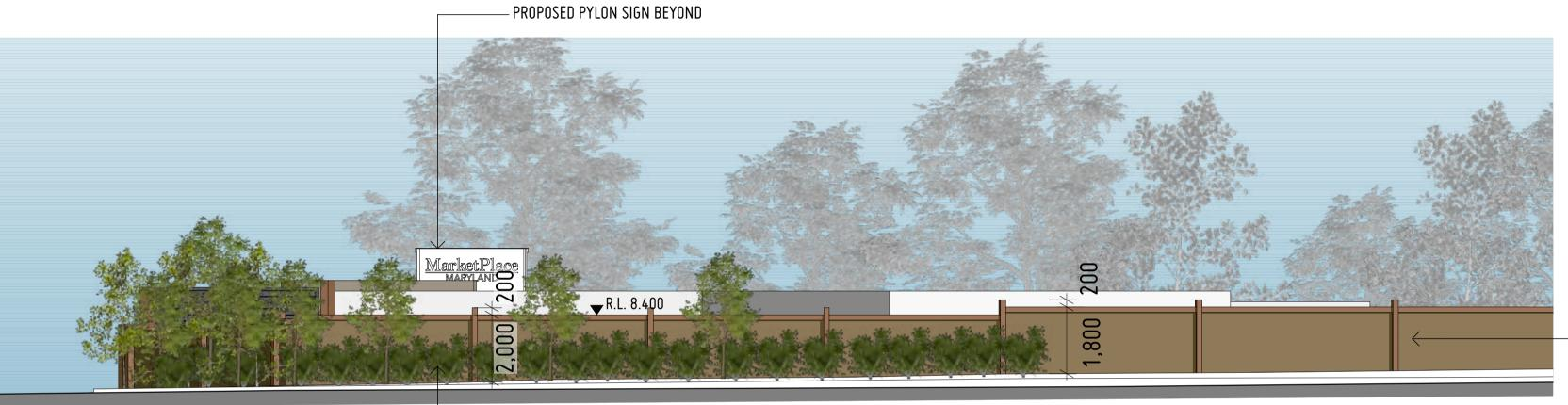
TIMBER CLAD ACOUSTIC WALL MAX. 2m TO MAIN BEER GARDEN
