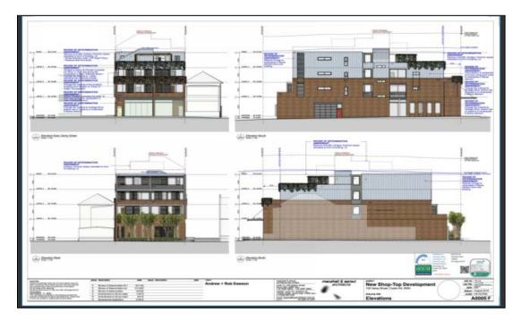
The building now has a much stronger emphasis on the two-storey built form of the ground and first floor. Clear separation is evident between the lower brick section and upper levels. The brick blade walls have been increased in thickness to anchor the building to the street and clearly define the two 'bays' of the façade. The composition of the façade fronting Darby Street is now more symmetrical with clearly defined 'bays' which reference the typical rhythm of the streetscape.
