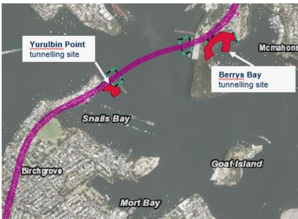
Figure 2: WHT tunneling sites nominated for unconfined sea disposal of terrestrial tunnel spoil
