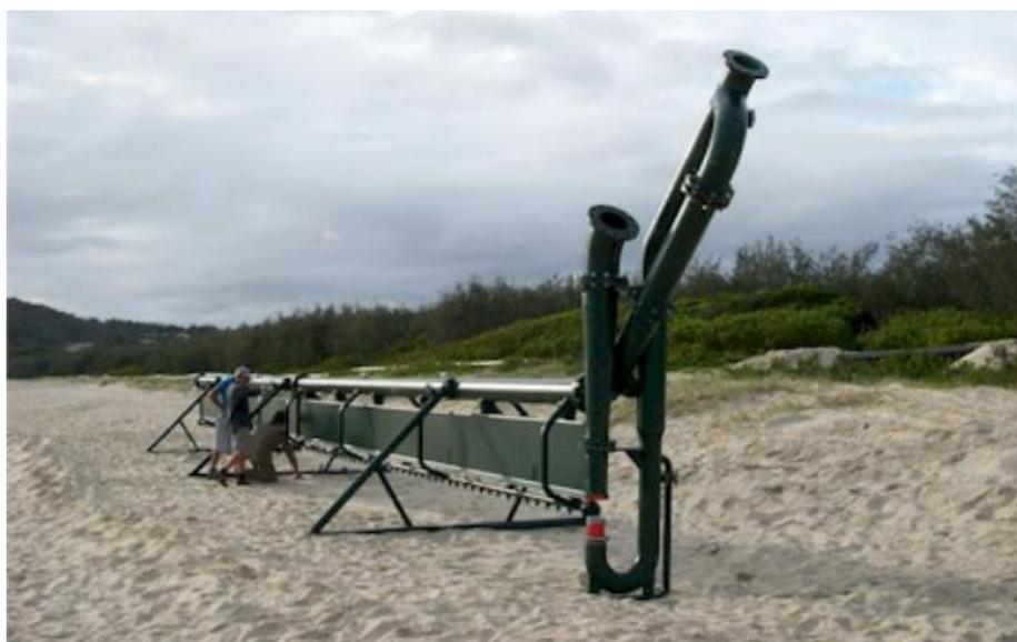
*Figure 4: Example submerged sand extraction unit*
