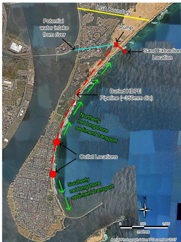
Figure 5: Sand backpassing schematic for Sand Shifter
