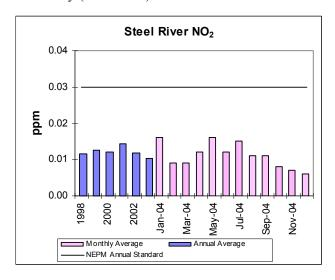
Graph 5: NO<sub>2</sub> Steel River Ambient Air Monitoring Station
