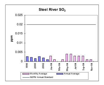
Graph 4: SO<sub>2</sub> Steel River Ambient Air Monitoring Station
